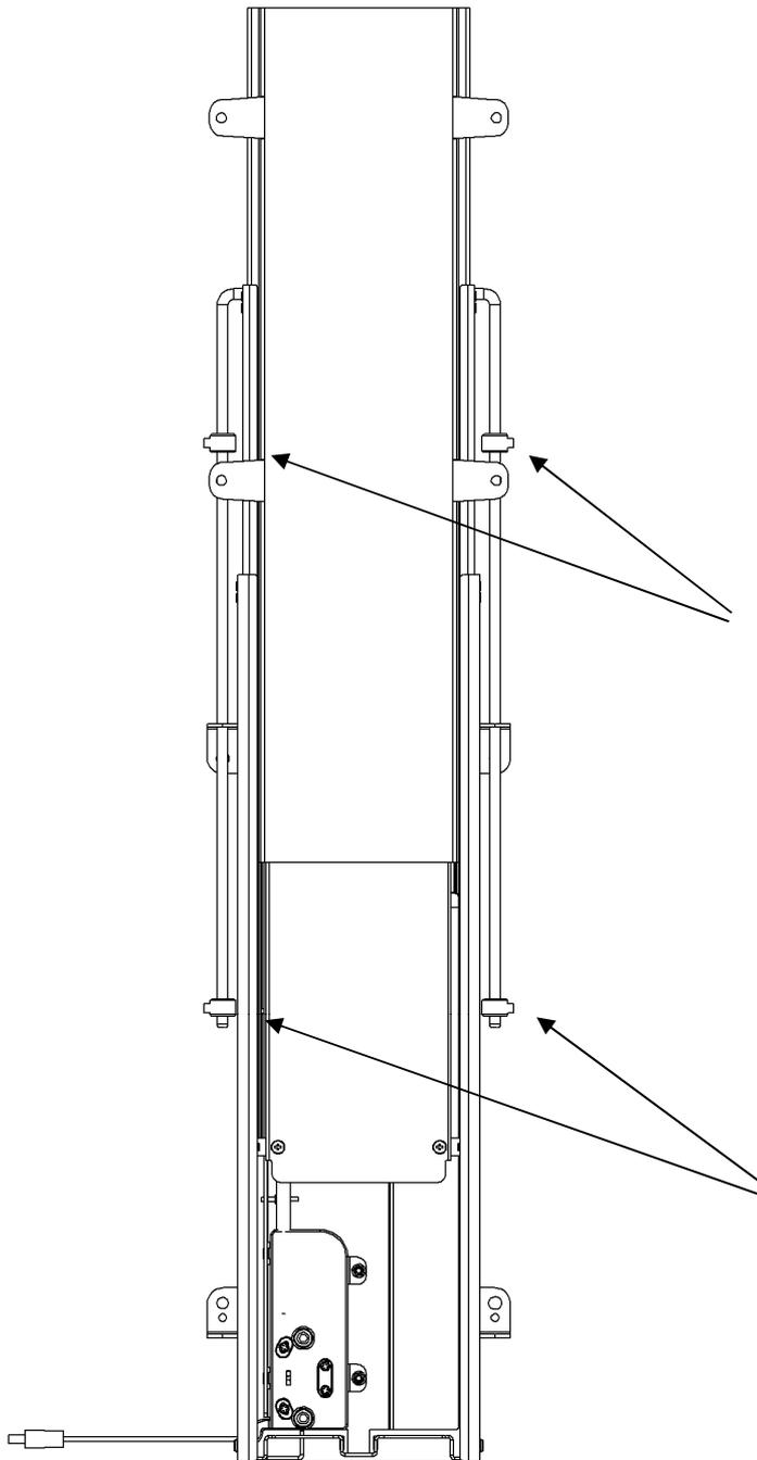
Adjust these 2 end stop sliders downwards to increase the height of the lifts lowest position. 2,5mm Allen key required. Make sure to tighten the screws properly.
